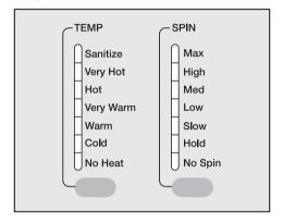
■ Press the "TEMP" and "SPIN" buttons until the indicator of the desired setting lights.
